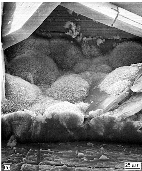
Figure 6 Scanning electron micrographs of nucleation layer on the PEEK surfaces with a thickness of about 10 \mu\text{m} and a spherulite-like shape (a). On the nucleation layer, crystallites with a rosette-like morphology were formed (b).
