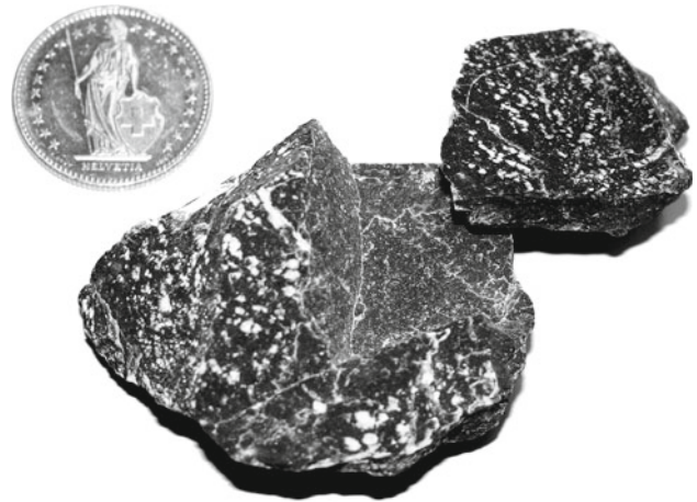
Fig. 4 Chunks of massive, micritic Malm limestone sampled from the sturzstrom of Flims. This sample is representative of the angularity of particles forming in sturzstroms—independent from their diameter and geology. The rough fracture surfaces are not pre-existent in the source rock but are newly formed by fragmentation during the transition of the sturzstrom. These two chunks fit together like a “jigsaw puzzle” [114, 115]. The white spots are lunette shaped impact marks by other rocks, but no signs of abrasion are observable (a 27 mm dia. coin serves as scale)
