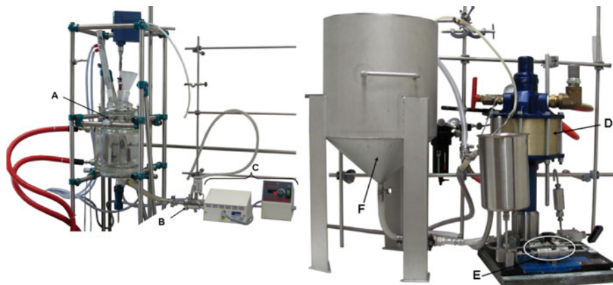
Fig. 2 Apparatus for cellulose disintegration, consisting of a reactor coupled to an inline disperser ( left ) and a high-shear homogenizer ( right ). a 10-L thermo-static reactor. b Ultra turrax. c Inline dispersing system. d Air pump. e Fixed-geometry interaction chambers (Y or Z morphology). f Container for NFC suspension
