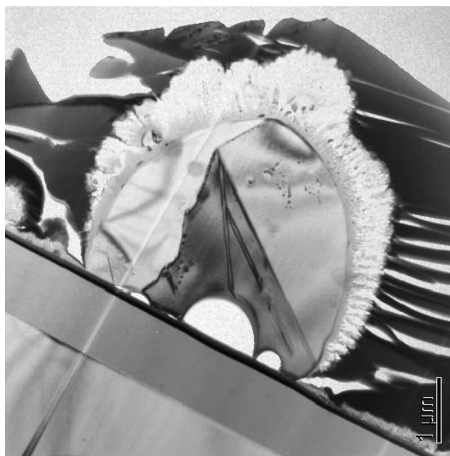
FIGURE 5 TEM lamella of a particle produced in helium that has trapped a gas bubble during settling. See text for description
