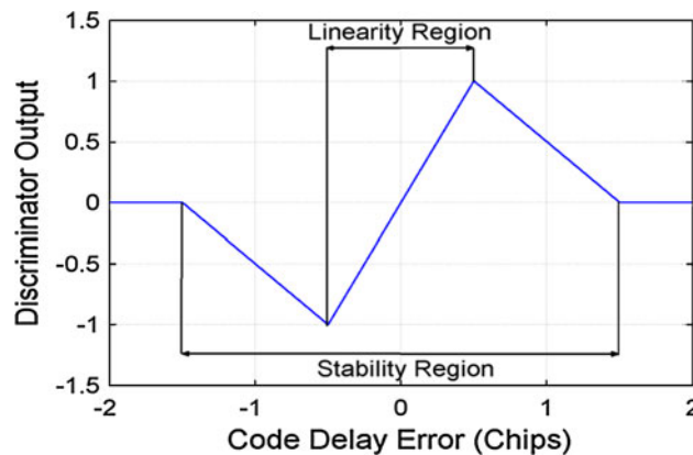
Fig. 7 Stability and linearity region for a typical discriminator output
