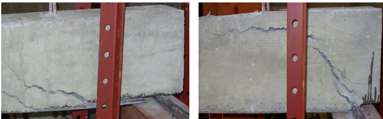
(a) Plate-end debonding
