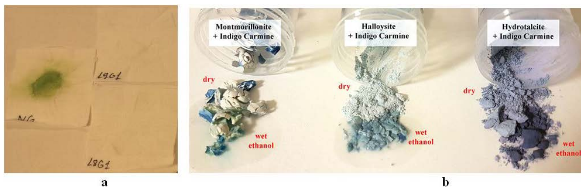
Figure 4. a) Cotton standard fabrics after wet rub test, with composite materials using epoxy bioresin and natural chlorophyll extract (NG), and hybrid pigments with lamellar nanoclays under different synthesis conditions. b) Hybrid pigments samples with indigo carmine and montmorillonite, or halloysite, or hydrotalcite nanoclay.
