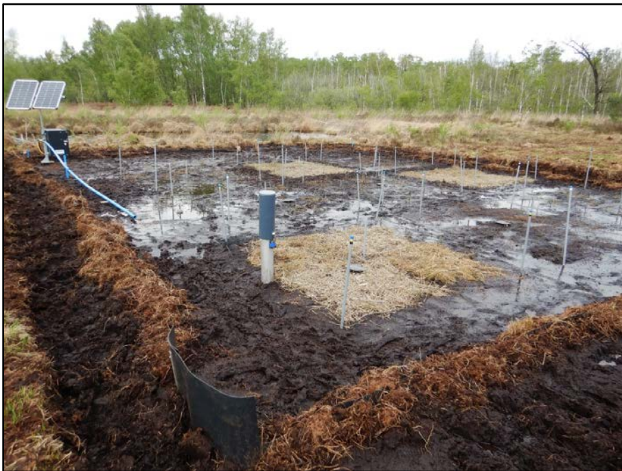
Photo of the experiment on bare peat in the Deurnsche Peel, where a solar pump is used to compensate for water losses. Picture by Hilde Tomassen.
