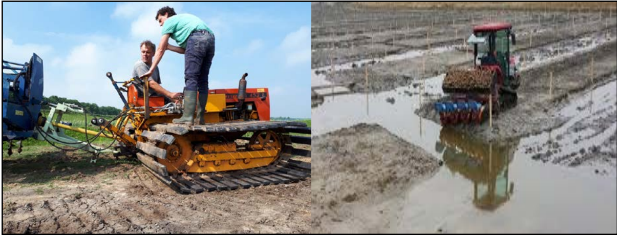
Figure 33. Planting machines developed for Typha (left; picture by Martijn Korthorst) and Phragmites rhizomes (right; picture by Gebr. Visscher).
