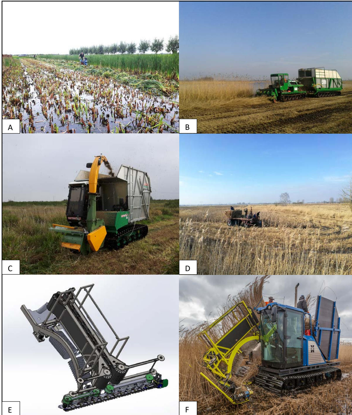
Figure 37. Harvesting machinery developed for biomass harvest in wet peatlands. Pictures by Jeroen Geurts, Hanze Wetlands, Christian Fritz and Tobias Dahms.
