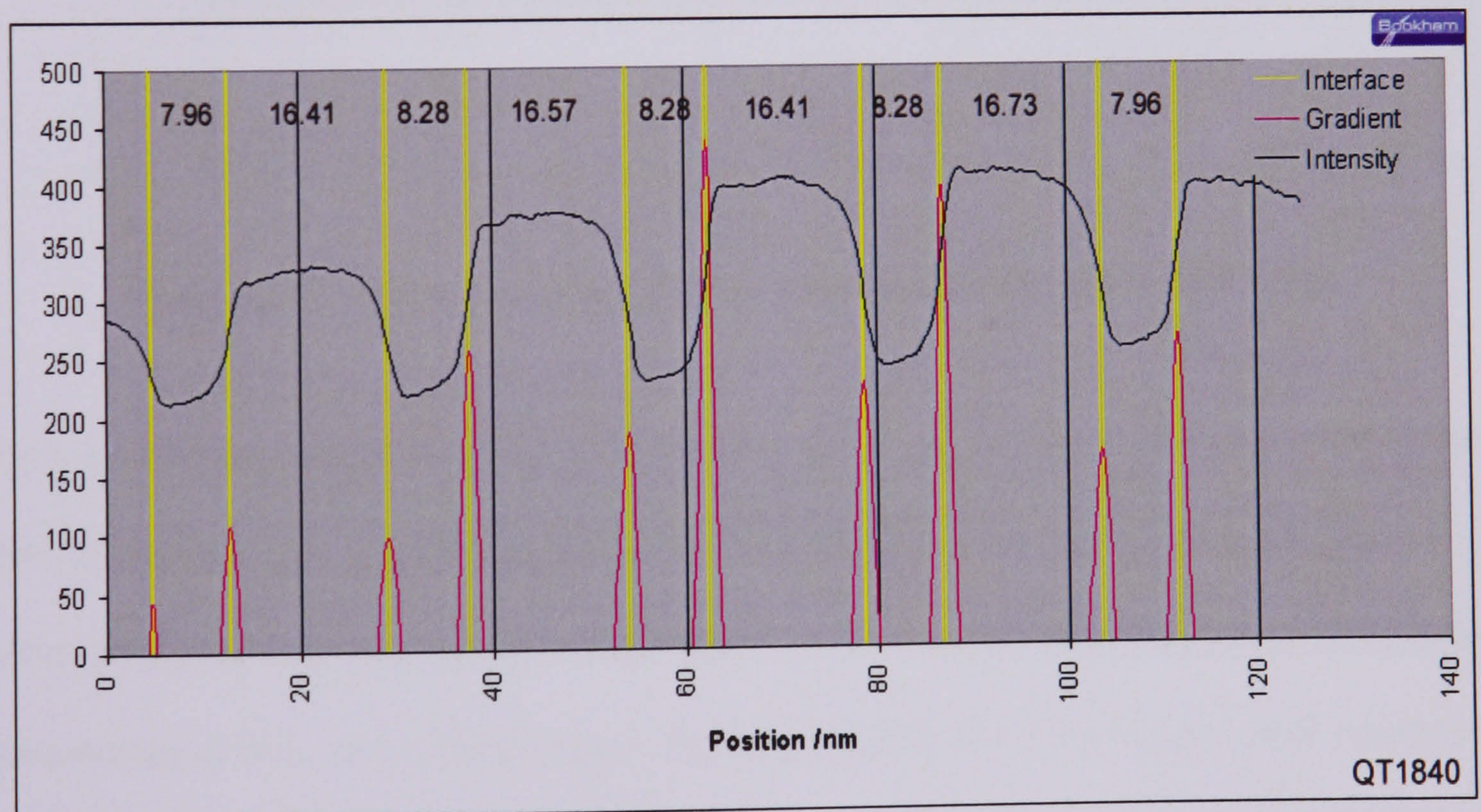
Figure 5.22 TEM and measured well and barrier widths for Qt1840
