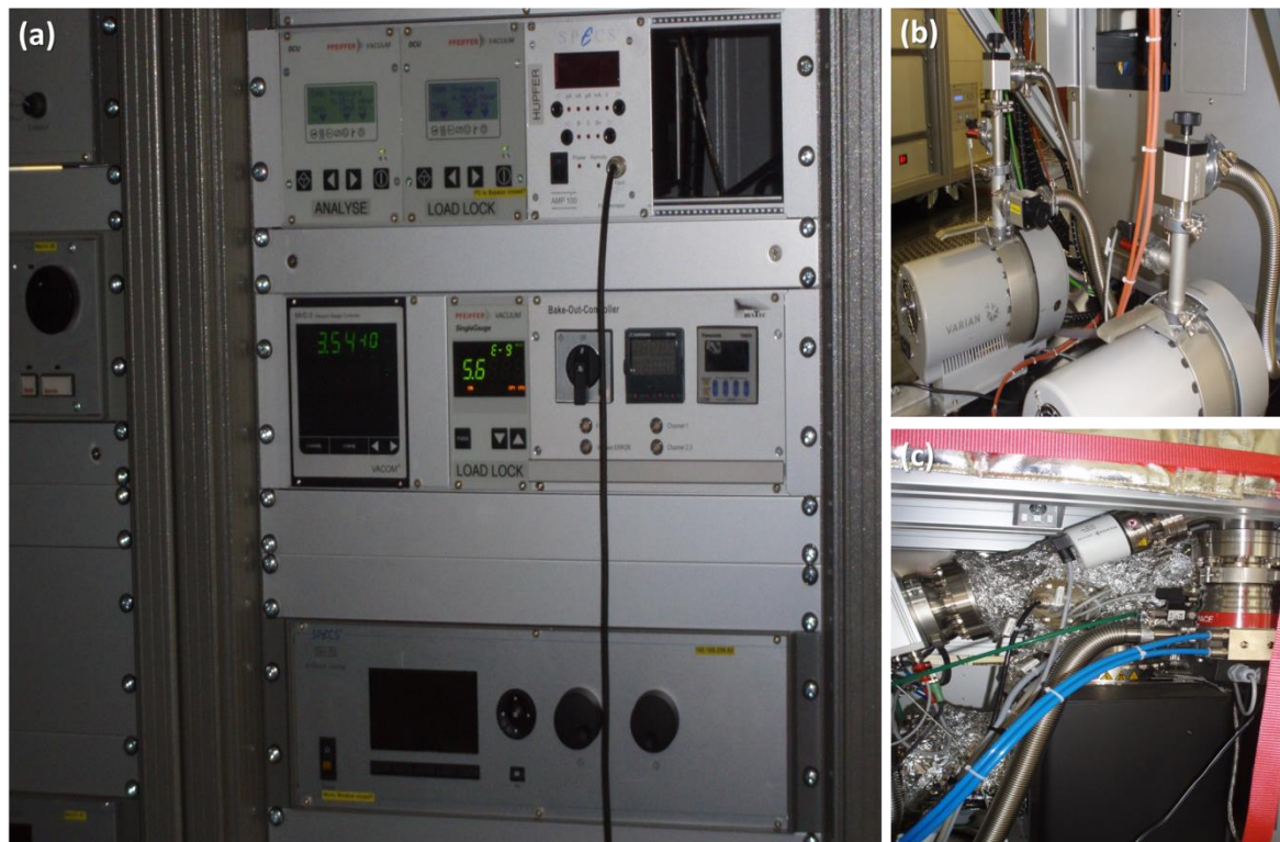
Figure 3-9: Base pressure (Ultra High Vacuum) achieved by using different pumps used. (b) Dry (oil free) rotary pumps, (c) Ion pump and titanium sublimation pump (TSP).
