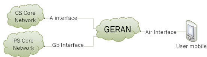
Figure 20 - Interfaces in GERAN core network (adapted from [19] and [28])
