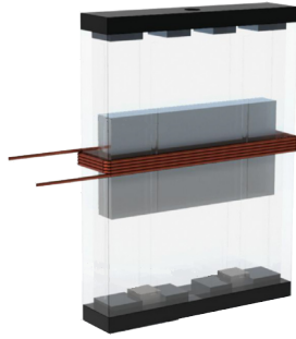
Figure 2.4: Box shaped magnetic levitation harvester proposed by Berdy et al. [6]
