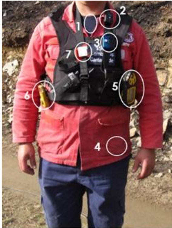
Figure 7 – Sensors attached to the firefighter clothes.
