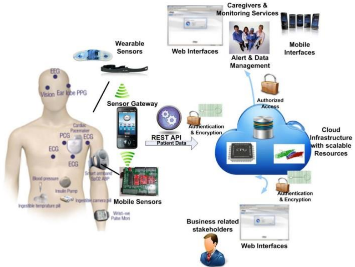
Figure 2 – Components architecture of a typical Internet of Things scenario [18].
