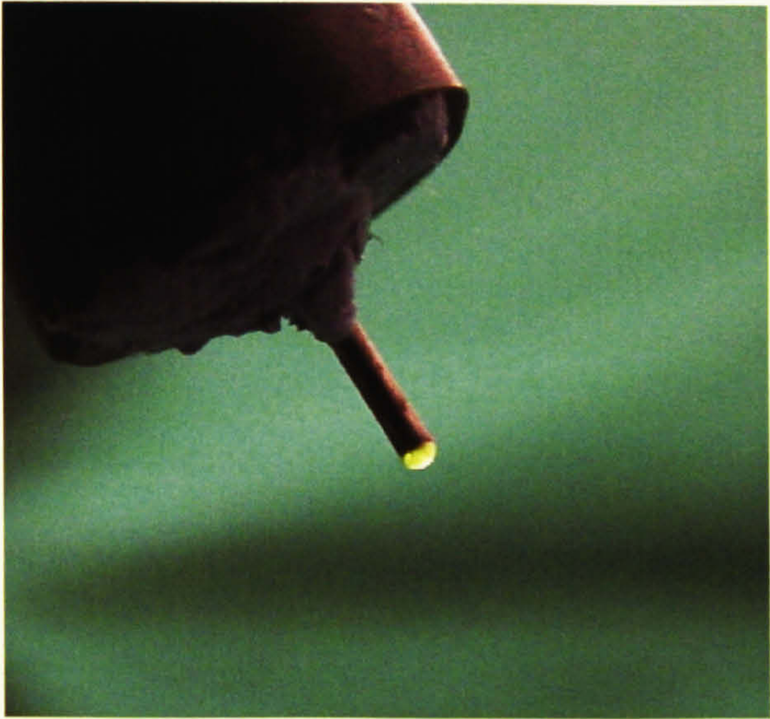
Figure 53 Tip of the optical fibre (with yellow phosphor) protruding from the 10mm steel tube
