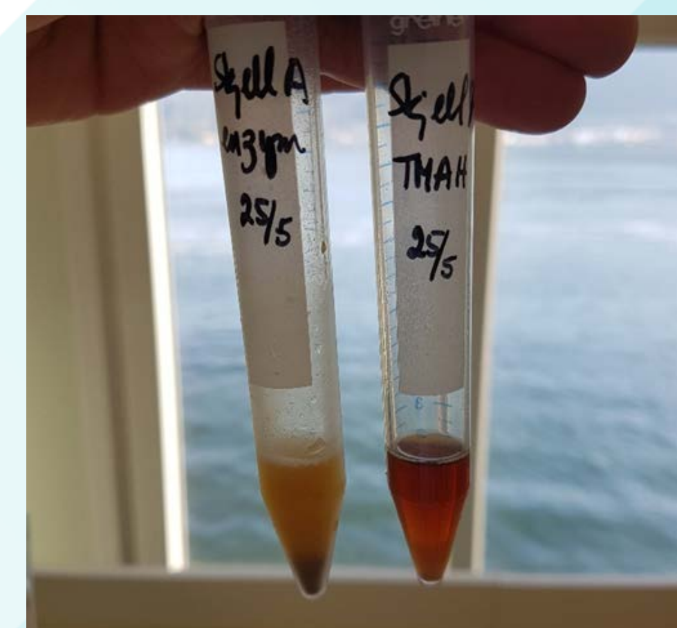
Figure 1. Sample digested with TMAH and enzyme (protamex). The TMAH extract was clearer compared to the enzymatic digest.
