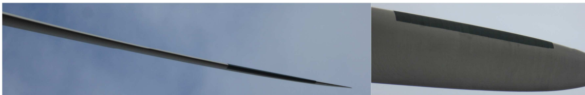
Figure 6. Roughness material installed on the blade
