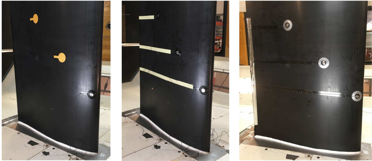
Figure 4. Sequence of microphones installation on the model.
