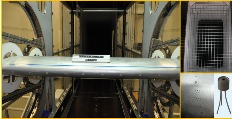
Figure 2. NACA 63-418 Airfoil in LM Wind Tunnel with bump tape(left), Turbulence grid(right-top) and Surface Microphones(right-bottom).
