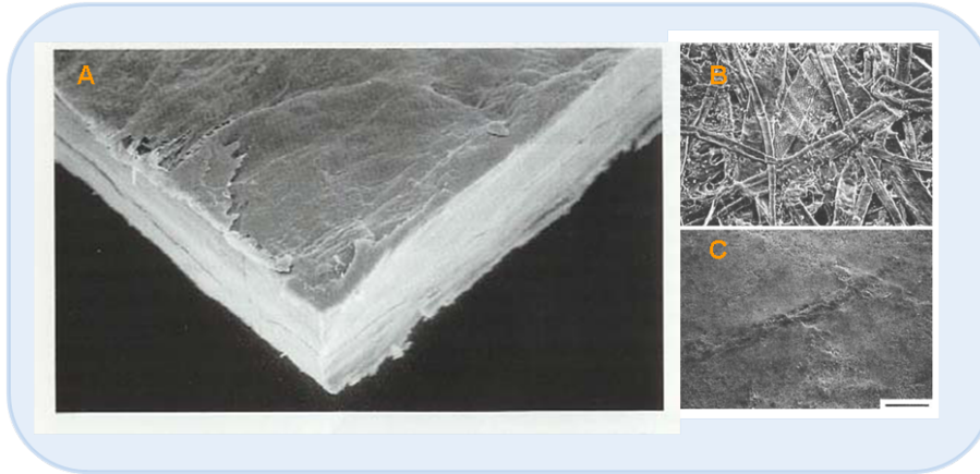
Figure 9: Environmental Scanning Electron Microscopy (E-SEM) picture of a greaseproof paper structure, showing the tightly sealed surface of the paper. The absence of macroscopic pores is due to extensive beating, which produces large amounts of highly hydrated fines and very collapsed fibre walls
