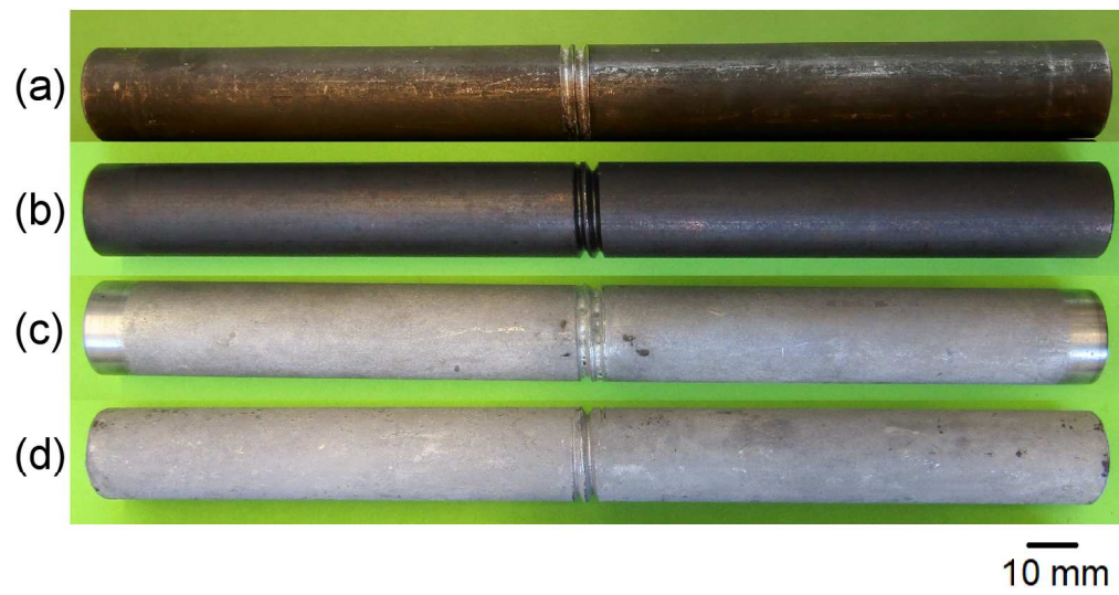
Fig 1 Representative samples used for tension-tension fatigue tests: (a) AM (uncoated thread) sample; (b) BO sample; (c) NTG sample; and (d) HTG sample.
