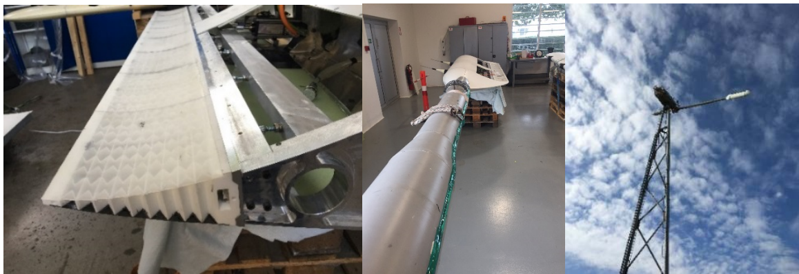
Figure 1. Left: The morphing flap mounted on the blade section, Centre: The blade section mounted on the rotating rig boom before installation. Right: The rotating rig with the mounted blade section.
