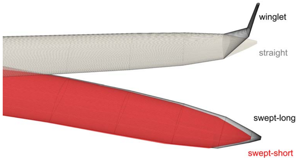
Figure 3: The four blade types investigated: straight (solid gray), winglet (wire-frame black), swept-short (solid red) and swept-long (wire-frame black).
