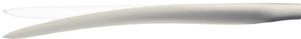
Figure 2: NREL 5 MW wind turbine blade with (solid) and without (mesh) sweep.
