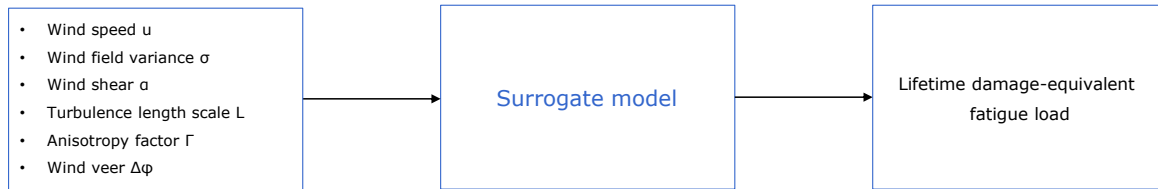
Figure 2. Schematic illustration of site-specific load estimation using surrogate model.
