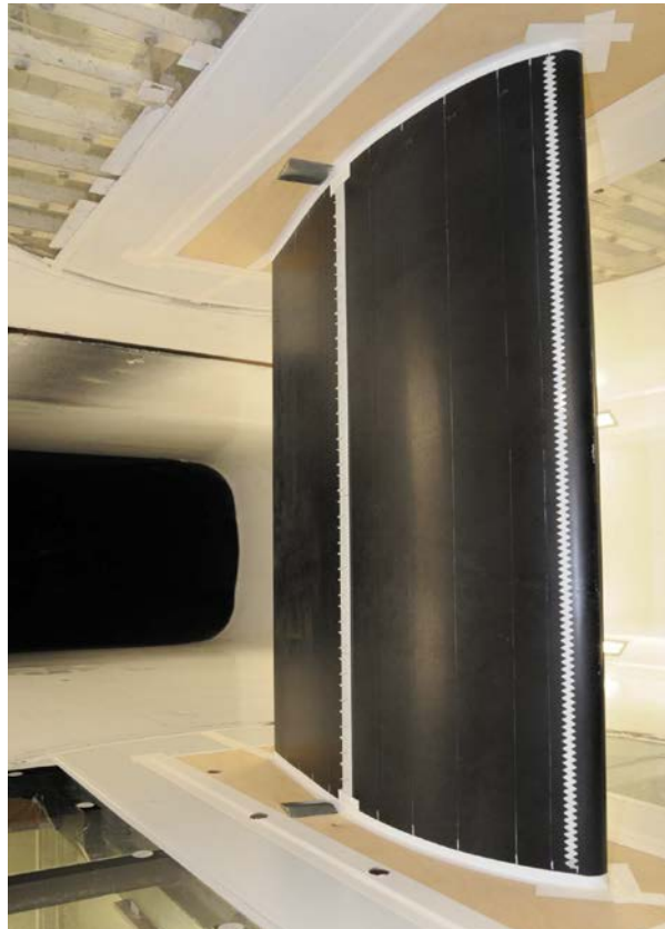
Figure 1 The NACA 63 3 -418 airfoil mounted in the test section with VGs and LER mounted at the surface.
