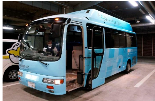
Fig.2.4 Microbus equipped with a 4.7 L 105 kW hydrogen engine
