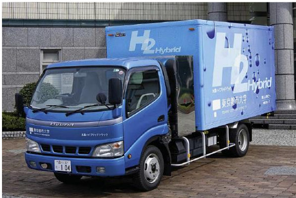
Fig.2.3 Hybrid light duty truck equipped with a 4 L 91 kW hydrogen engine
