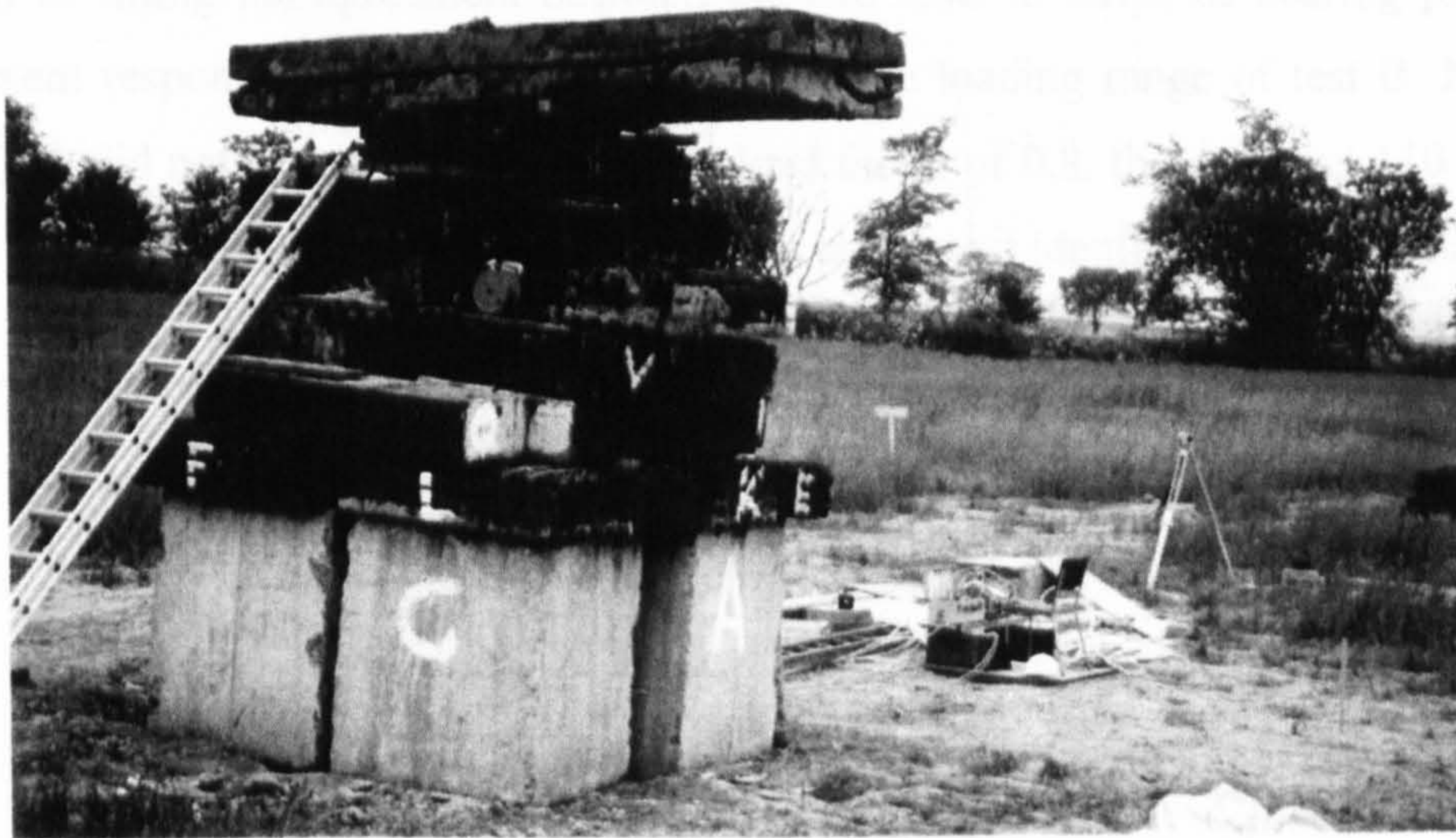
Figure 8.18: Footing A at failure (after Gildea, 1990).
