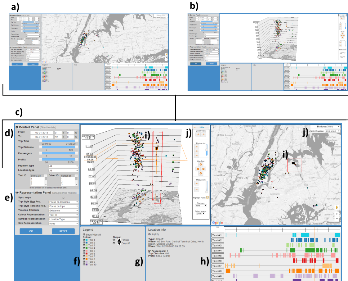
Figure 5.1: TTV prototypes a) 2D map prototype; b) STC prototype; c) 2D map + STC prototype; d) Control panel; e) Representation panel; f) Legend; g) Information panel; h) Timeline; and i) Spatial highlight reflected in both maps.
