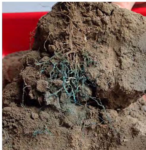
Figure 5. Tracer test with Brilliant Blue FCF shows the uptake via roots when irrigating from the bottom.
