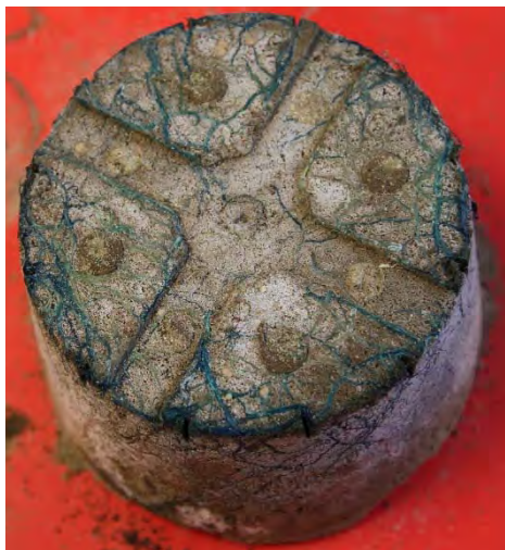
Figure 5. Tracer test with Brilliant Blue FCF shows the uptake via roots when irrigating from the bottom.
