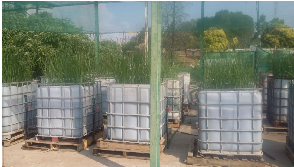
Fig. 1 Experimental setup showing pipe connections with V. zizanioides in VFCW
