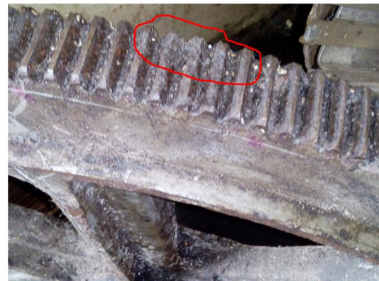
Plate 1: Pictorial view of the failed teeth of a spur gear during an operation
