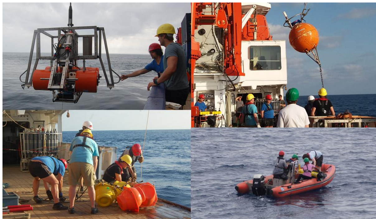
Fig. 1: Deployment of a lander (upper left), recovery of a long-term mooring from the continental slope at 11°S (upper right and lower left) and the recovery of an ocean glider after successfully completing its mission (lower right).
