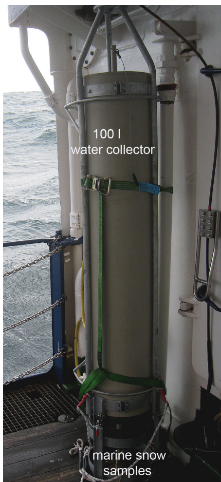
Fig. 3.1 The Marine Snow Catcher (MSC) on board of R/V Poseidon. The water volume sampled by the collector is 100 l. Marine snow particles settle downwards into a collector where they can be sampled.
