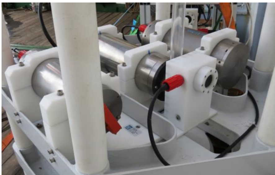
Fig. 3.6: The Camera System on the BOP with the camera housing in the middle (for camera, lens and system electronics), the VIS light source and the Li-ion battery.
