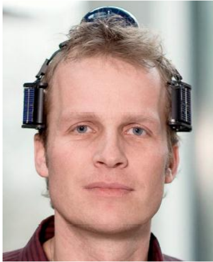
Figure 2.8: Body-powered EEG headband; TEG and PV cells (Yazicioglu et. al., 2008)
