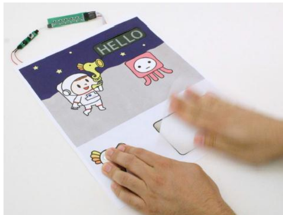
Figure 2.14: Human heat energy harvesting through hand rubbing and display on electronically in paper (Karagozler et, al, 2013)
