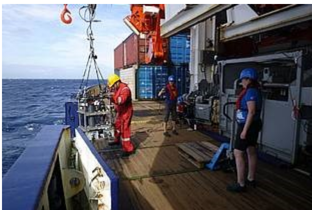
Fig. 1: Optical sensor package before deployment. (Photo: Katrin Hessner)
