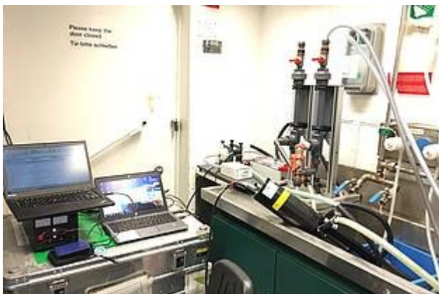
Fig. 3: Continuous measurement of the scattering and absorption properties with an ACS photometer in the sea water circulation system. (Photo: Hongyan Xi)
