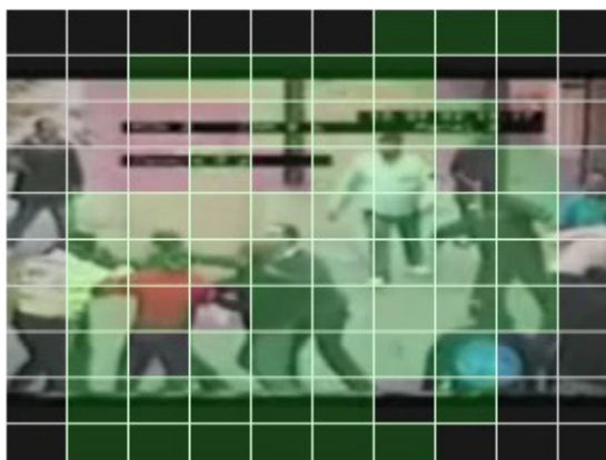
Fig. 2. Crowd density calculation grid for a scene from the violent-flows dataset. Each green square corresponds to an occupied grid cell (crowd density in this frame = 57%).
