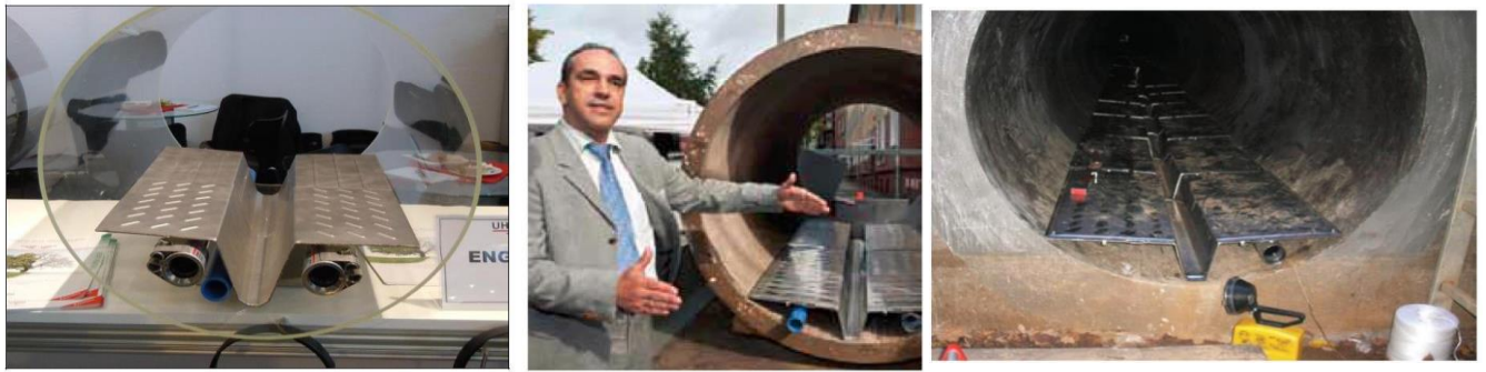
Figure 13 - 15: Modular Plate Heat Exchangers (Cipolla and Maglionico 2014; Hamburg Wasser 2012; Pamminger et al. 2013)
