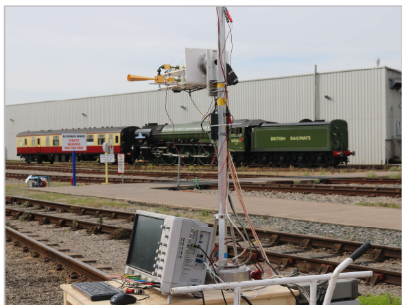
Fig. 2. Receiver architecture using orthomode transducer, Keysight MSOS804A 20 GHz oscilloscope and 89600 VSA software interface.
