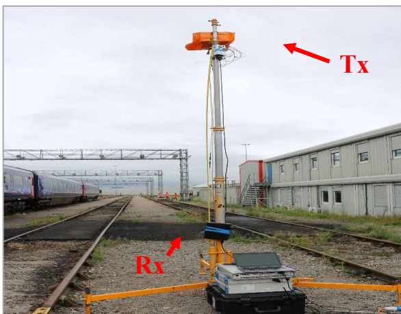
Fig. 1. 60 GHz transmitter setup using Keysight M8190 AWG and SiviersIMA, and the measurement scenario.
