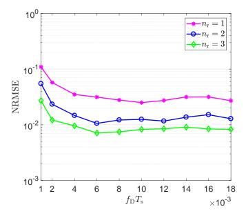
Fig. 7. The effect of  $n_{\rm r}$  on the performance of the proposed NDA-MBE for  $n_{\rm t}=2$  and at  $\gamma=10$  dB.
