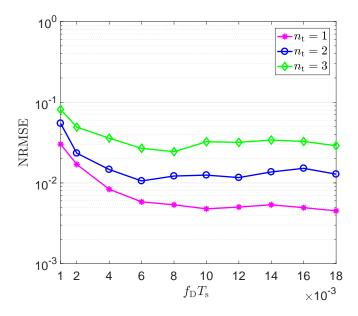
Fig. 6. The effect of  $n_{\rm t}$  on the performance of the proposed NDA-MBE for  $n_{\rm r}=2$  and at  $\gamma=10$  dB.
