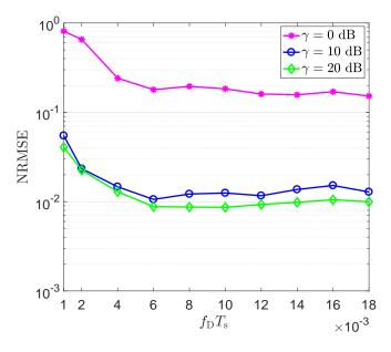
Fig. 5. The NRMSE of the proposed NDA-MBE versus  $f_{\rm D}T_{\rm s}$  for different SNR values.
