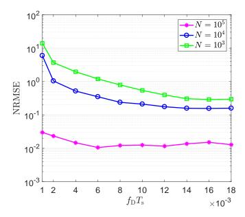
Fig. 9. The effect of the observation window size, N, on the performance of the proposed NDA-MBE for  $n_{\rm t}=2$  and  $n_{\rm r}=2$  in frequency-selective channel, and at  $\gamma=10$  dB.
