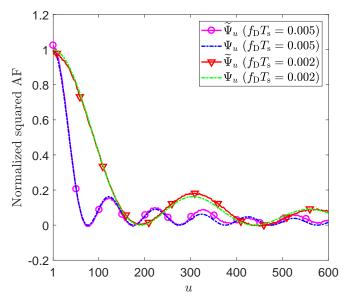
Fig. 1. Illustration of the non-linear LS regression for the uniformly sampled normalized squared AF for  $f_{\rm D}T_{\rm s}=0.02$  and  $f_{\rm D}T_{\rm s}=0.005$ , with  $n_{\rm t}=1$ ,  $n_{\rm r}=2$ , L=1,  $u_{\rm s}=2$ , and at  $\gamma=10$  dB.
