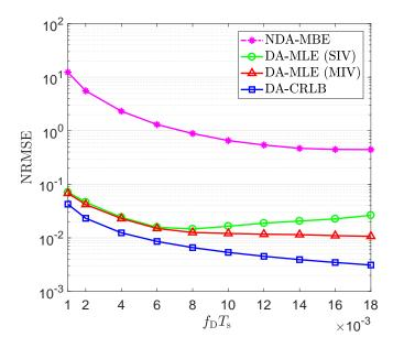
Fig. 11. Performance comparison of the proposed NDA-MBE, the derived DA-CRLB, and the derived DA-MLE (SIV and MIV) in MIMO frequency-selective Rayleigh fading channel for  $n_{\rm t}=2,~n_{\rm r}=2,~L=5,~N=10^3,$  and at  $\gamma=10$  dB.
