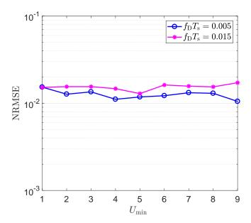
Fig. 8. The effect of the parameter  $U_{\min}$  on the performance of the proposed NDA-MBE for different values of  $f_{\rm d}T_{\rm s}$  and at  $\gamma=10$  dB.
