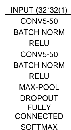
Figure 3: CNN Architecture with 2 convolutional and 2 max-pool layers.
