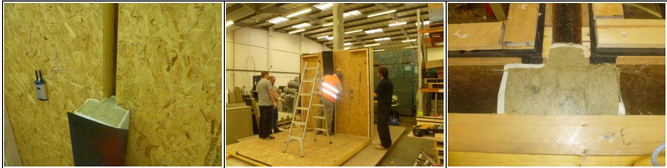
Figure 42 Test 4.12, ARC T-Barrier, 75 mm party wall, 150 mm external wall
