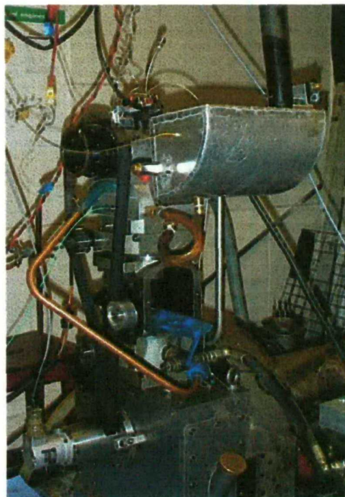
Figure 3.2: Photograph of optical single cylinder engine
