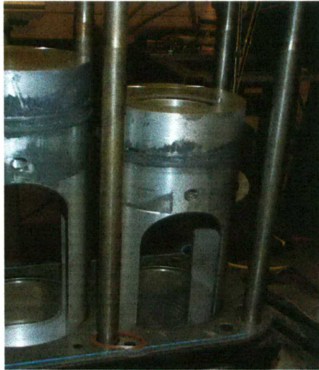
Figure 4.3: Optical piston protruding from original block
