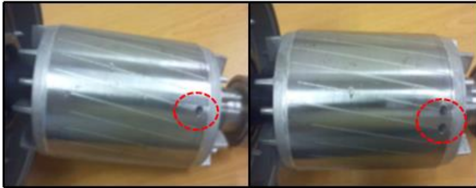
Figure 5.10 Rotor with one and two broken bars
