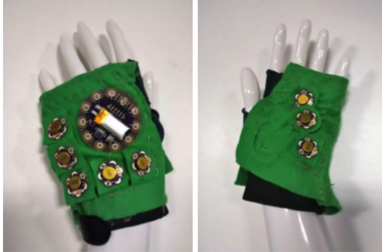
Figure 4.1: Glove prototype 4. Left: back, right: palmar of the glove.
