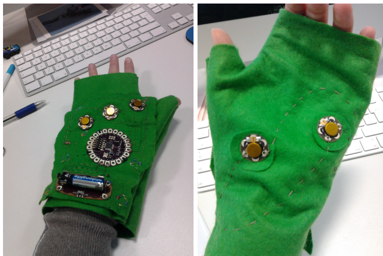
Figure 3.8: Glove prototype 3. Left: front, right: back of the glove.
