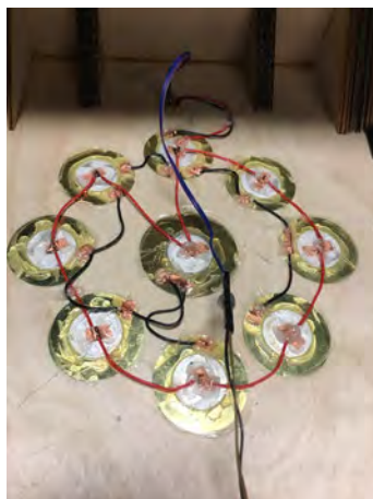
Figure 6.8: A piezo network in a large MOAI. Piezo discs are 50mm in diameter, connected in parallel, and the slider joints are insulated and protected with hot glue.
