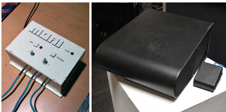
Figure 6.2: Left: The MOAI control interface. Right: A large MOAI element and a small MOAI element, illustrating the difference in size (Large, 40x30x20cm; small, 12x10x5cm).
