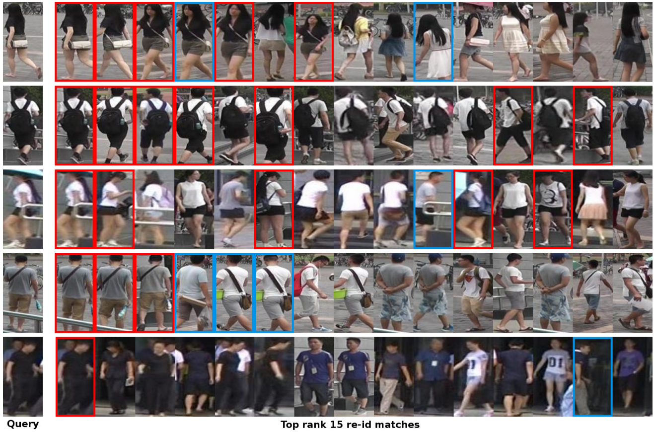
Figure 8. The top 15 re-id matches by the DLDP model on the Market-1501 dataset. Correct matches are framed red. Matches labelled as “junk” in the dataset and not considered in the evaluation protocol are framed blue. The last row shows a failure case where only one (out of five) correct images could be found in the top 15 results.
