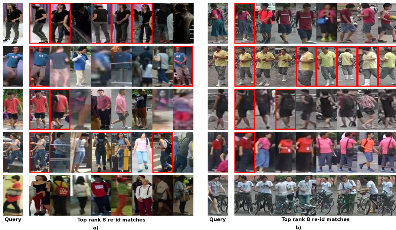
Figure 4. (a) The top 8 re-id matches by the DLDP model on the CUHK-SYSU test data for a set of five randomly chosen queries from the 100 image gallery setting, and (b) five randomly chosen queries on the PRW test data. Note, rank-2 and rank-3 in the “yellow T-shirt” example in (b) are false matches even though they look very similar. The bottom examples from both (a) and (b) show failure cases when the model failed to find a match in the top 8 ranks.
