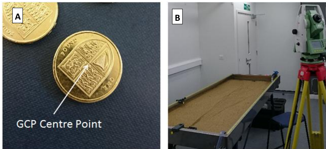
Figure 5.3 A) The GCPs used within the flume within this study. The cross hair of the shield was identifiable from the Total station as well as within imagery captured of the flume B) Total station used to provide referencing of the GCPs within the flume.
