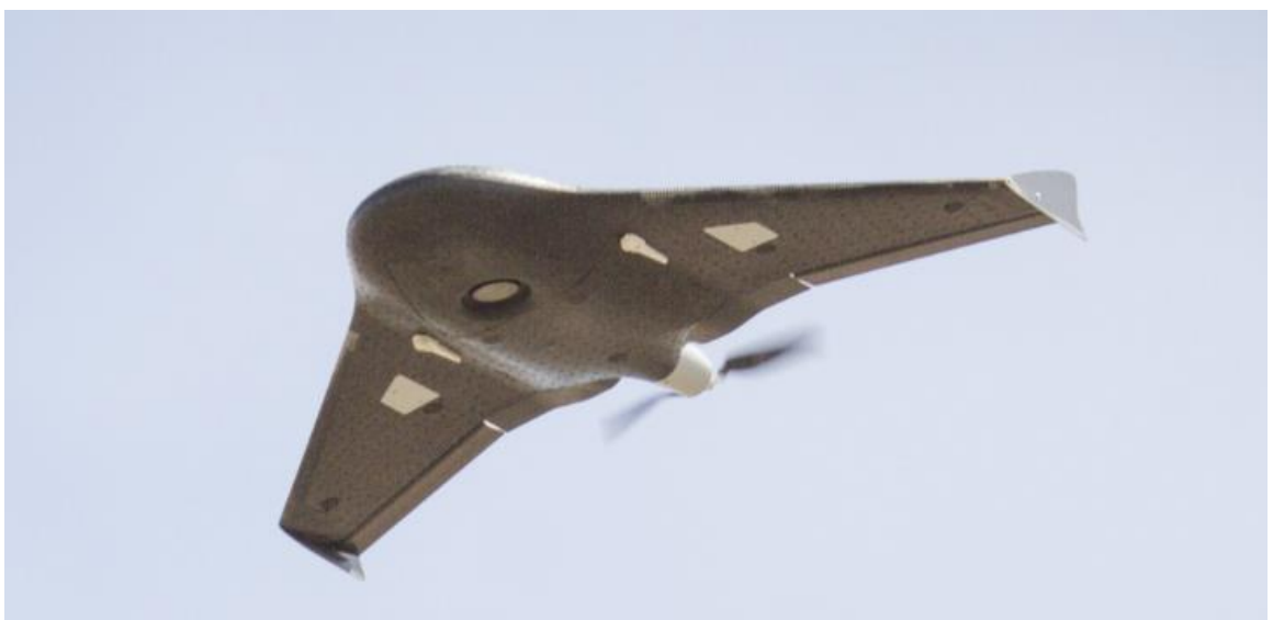
Figure 3.19 Trimble UX5 fixed wing UAS with range of 60 km and max flight time of 50 minutes.
