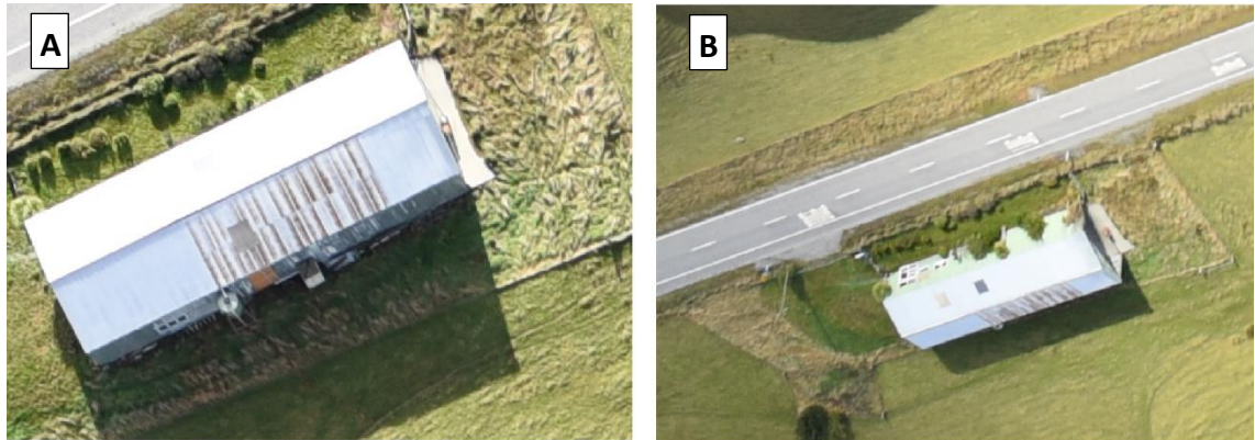
Figure 6.23 Imagery captured from the catchment wide scan of the barn, highlighting the issues faced during the dense pixel based matching stage. The high exposure in (A) results in a lack of features on the barn roof observed in (B).
