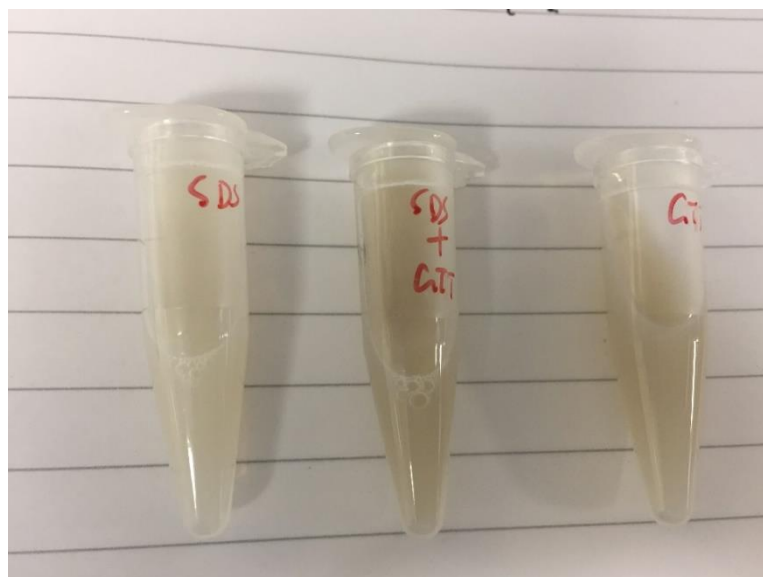
Figure 6-8 Dispersion of BNNTs in (from left to right): SDS surfactant solution, SDS-DNA solution, DNA ((GTT) 3 G) solution.
