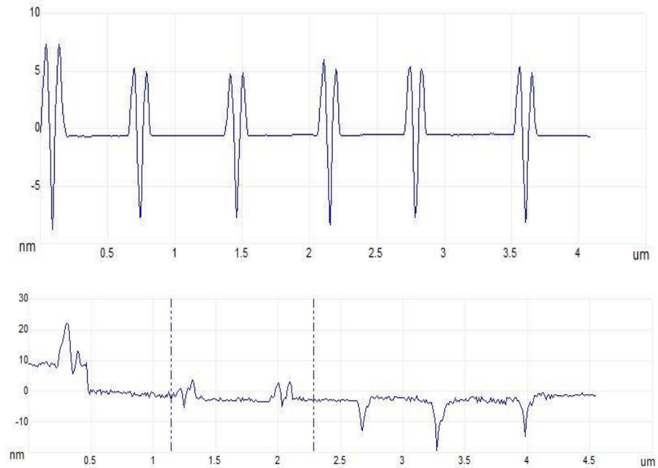
Figure 5-16 Topographical profiles obtained from AFM topographical images of the trenches : Upper, cross section image of sample from left sample in Figure 5-15 ; bottom, cross section image of right sample in Figure 5-15 .
