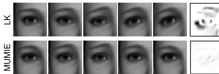
Figure 3.2: Illustration of drift errors that can occur over time, through an exemplar sequence that starts and ends with the same eye expression. Registration output of a Lucas-Kanade (LK) method [233] (top) and MUMIE (bottom). LK is prone to drift errors, as seen by comparing the first and last frames of the registered sequences. Drift errors are highlighted in the last column where the difference between the first and last frames is depicted. (Dark values indicate registration errors.)
