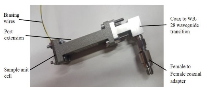
Fig. 3 Experimental setup for the unit-cell characterisation
