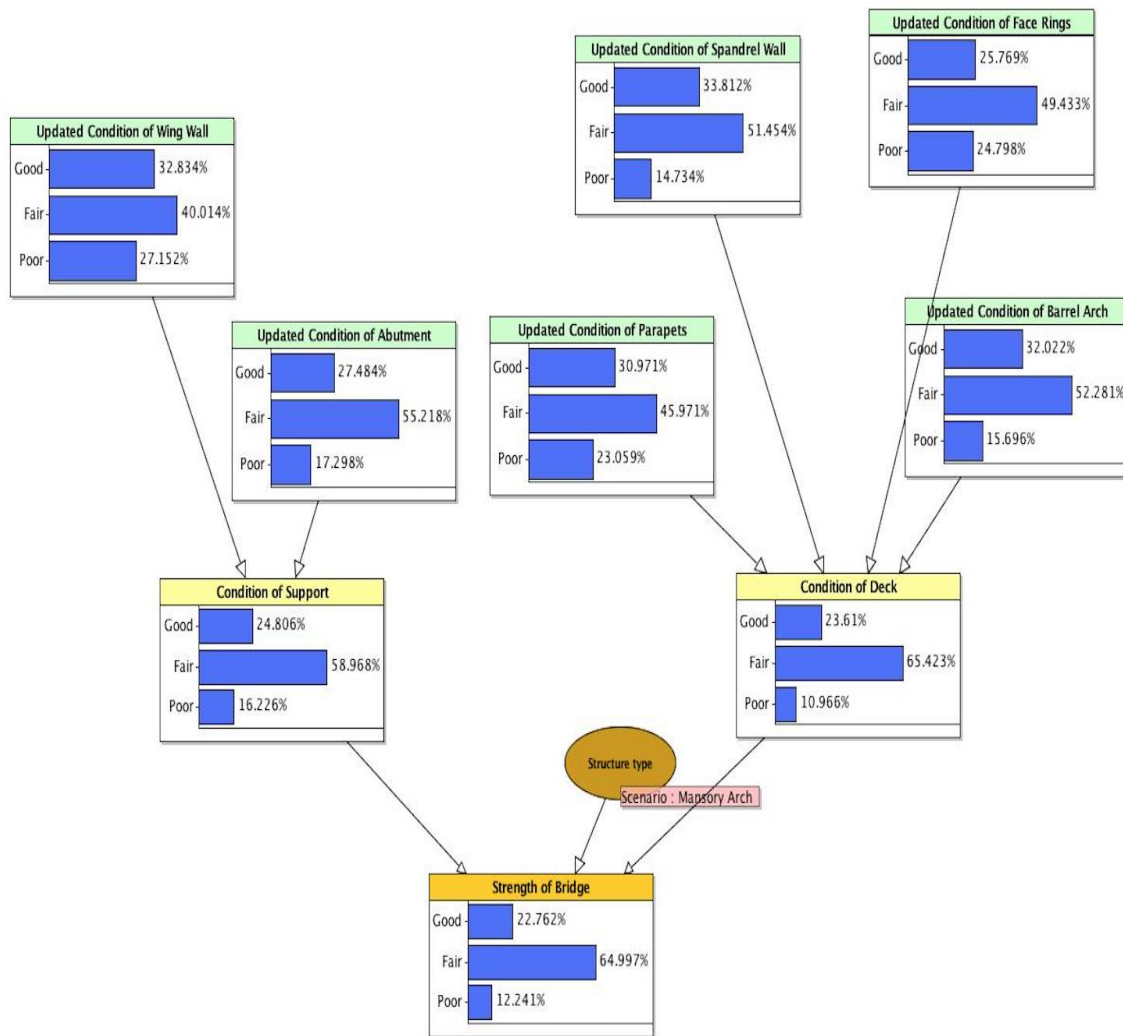
Figure 12. Strength of a typical masonry arch bridge.
