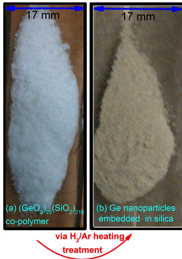
Figure 2.2.3.3 Picture of samples produced using the sol-gel method: (a) (\text{GeO}_2)_{25}(\text{SiO}_2)_{218} co-polymer (b) Ge NCs embedded in silica matrix. The pictures were taken using an HTC Desire HD cellular phone. Pale brown sample in (b) may be considered as an indication for the formation of Ge nanoparticles.
